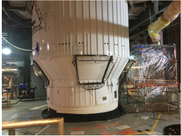
Fig. 26 OSIRIS-REx fairing “boat tail” doors and one clean tent are nearly ready to be removed for final closeout
